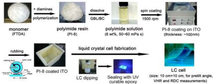
Figure 12. LC cells fabrication procedure from monomer synthesis to devices
