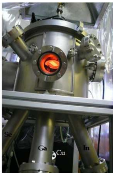
Fig. 8. Thermal co-evaporation system with Knudsen effusion cells to deposit Cu(In,Ga)Se 2 thin films
