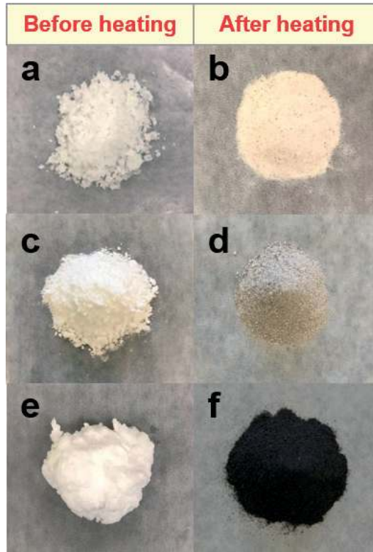
Figure 1. Image of synthesized \text{SiO}_x composite prepared using \text{SiCl}_4 and water (a and b), \text{SiCl}_4 and ethanol (c and d), and \text{SiCl}_4 and ethylene glycol (e and f) respectively.
