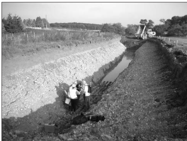
Fig. 2.53. Ripon North: sampling for OSL and clast analysis from Section 1, in the temporary trench near Norton Mills Farm.
