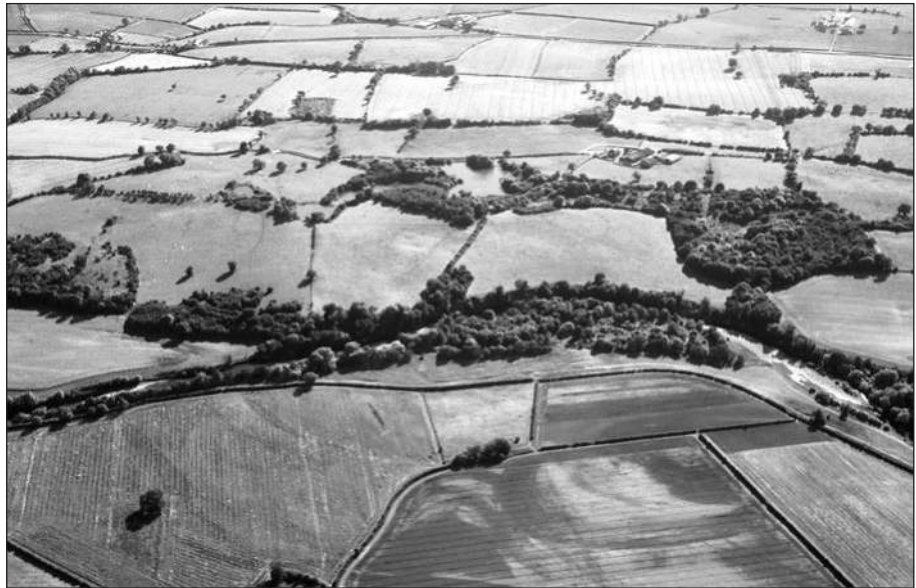
Fig. 2.24. Aerial view of Queen Mary's Dubb, north of Ripon (see Fig. 2.19); these pools are solution hollows within Permian gypsum just north of Ripon. Also note the clear field markings showing meander cut off patterns on aggradational terraces on the east side of the River Ure.
