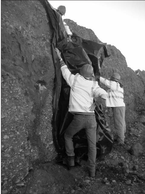
Fig. 2.1. OSL sampling at Nosterfield Quarry. In order to extract sand grains from gravelly deposits, into which a tube could not be driven, it was necessary for Helen Roberts to undertake the sampling behind a black PVC sheet. See section 2.6.2.
