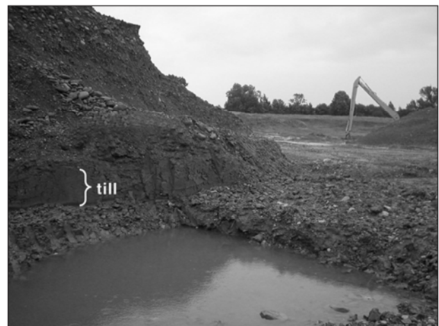
Fig. 2.61. Catterick quarry: view of working face, showing till overlain by the lower and upper gravels illustrated in Figure 2.60B.
