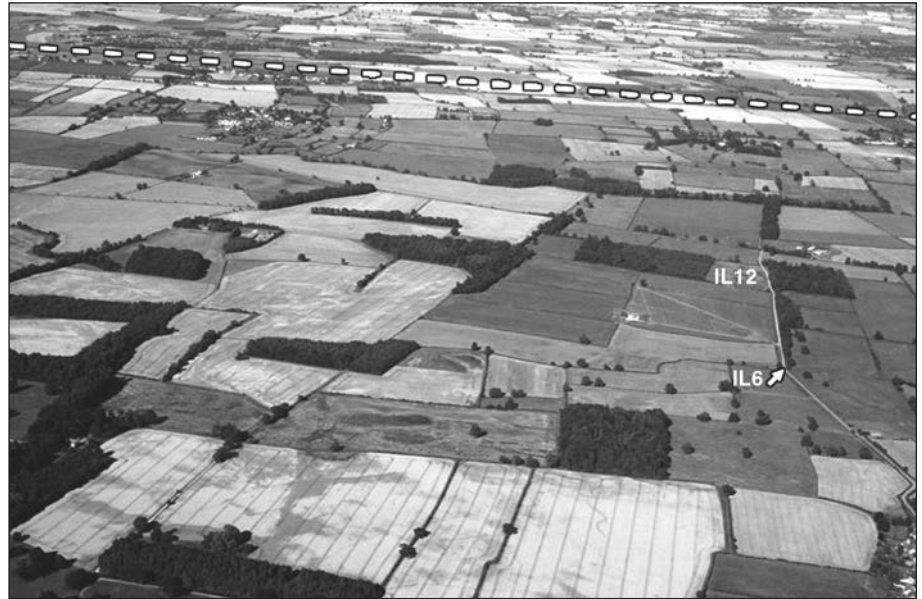
Fig. 2.31. Aerial view looking east across Snape Mires towards the A1 (dashed line). The low-lying area is underlain by thick (>18 m) lacustrine silts and clays deposited in a former glacial lake. Two of the palaeoenvironmental sample locations (see Chapter 3) are indicated.
