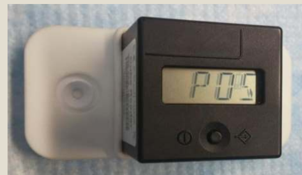
Fig. 2. opTricon Cube-Reader placed over the LFA device
