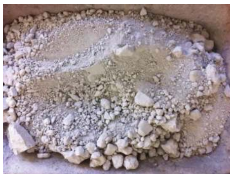
Figure 4. CSF as received (with 42% moisture content).
