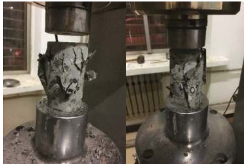
Figure 16. Typical failure modes of FRC under a dynamic load.
