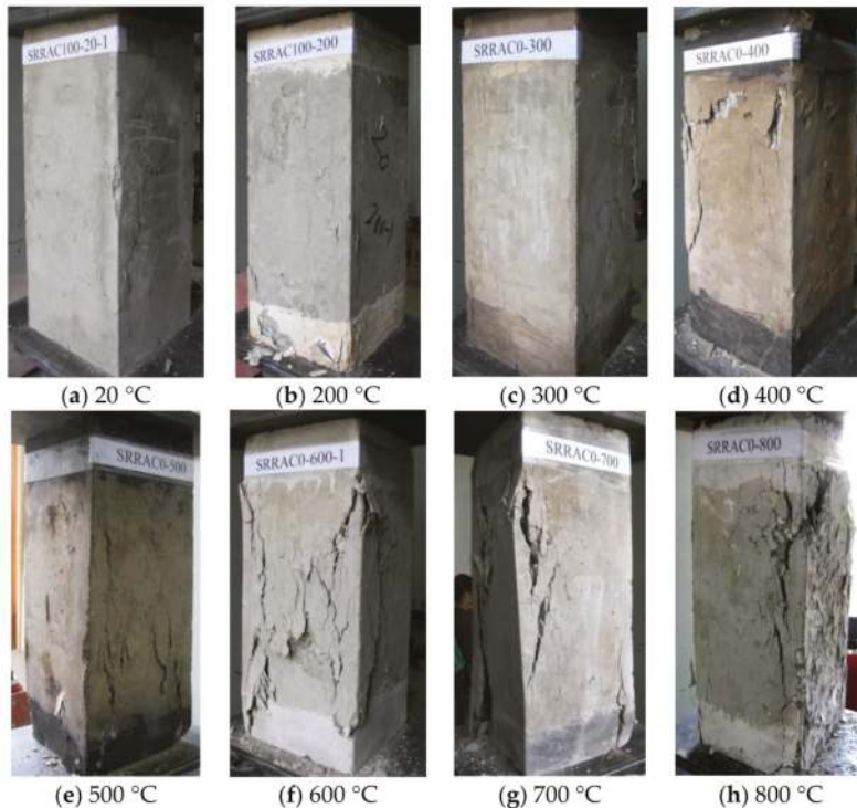
Figure 8. The failure modes of column specimen.
