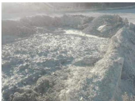
Figure 3. Stockpiled cement sludge fines (CSF) within the ready-mixed concrete (RMC) plant.
