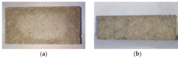
Figure 7. Front and side faces of one concrete paving block. (a) plan view of a concrete paving block; (b) lateral view of a concrete paving block.
