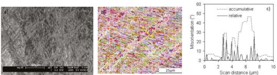
Figure 5. Characteristic features of shear bands formed in the 2nd pass; (a) FEGSEM backscatter image; (b) EBSD map and (c) a linescan of relative and accumulative boundary misorientations along ab in (b), demonstrating the generation of medium and high angle boundaries by shear banding.
