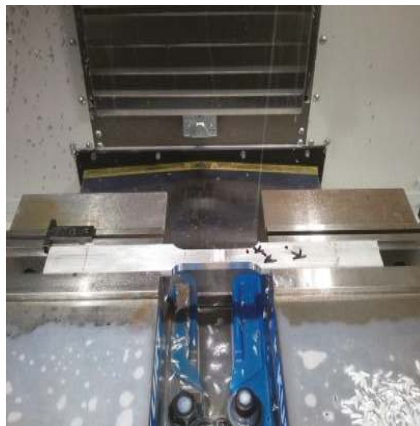
Figure 2. A finished tensile test specimen containing a fillet weld subsequent to machining on a Computer Numerical Control (CNC) machine.
