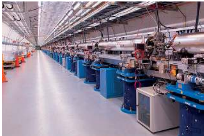
Figure 1. Schematic of the 33 m long LCLS FEL undulator [34].
