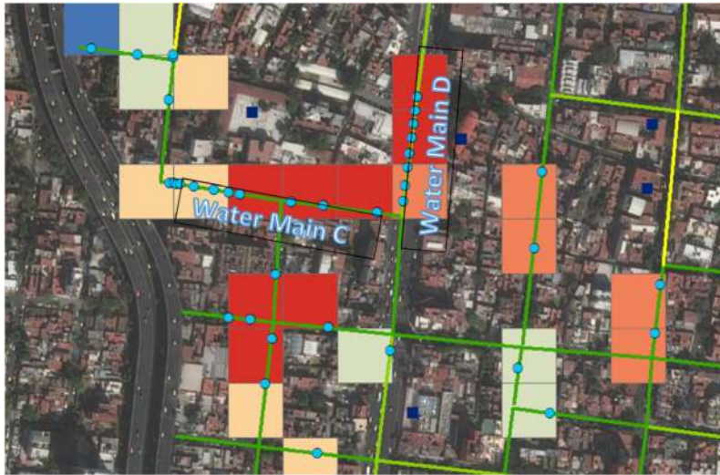
Figure 14.50 Example of COF/LOF analysis for two water mains (refer to online version of the book to visualize colors).
