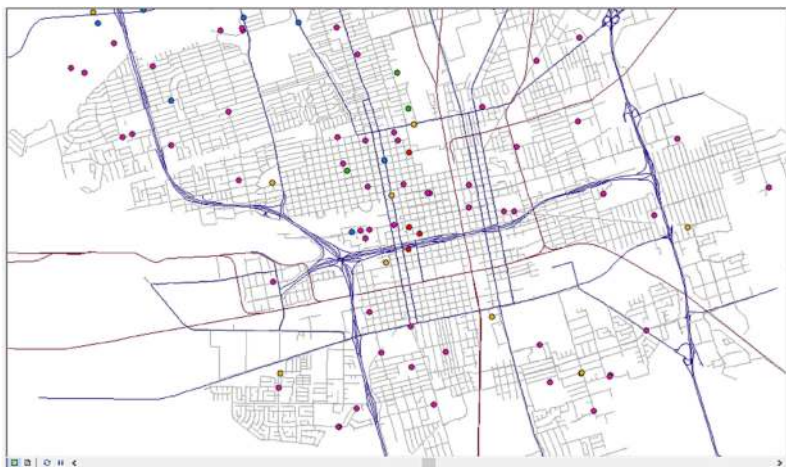
Figure 14.16 Critical facilities shapefiles. Dark lines represent highways and railroad tracks, dots represent critical infrastructure and light gray lines represent water mains.
