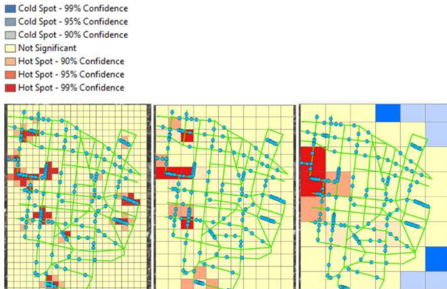
Figure 14.32 Hot spot analysis tool results with bin sizes of 50, 100 and 200 m (refer to online version of the book to visualize colors).
