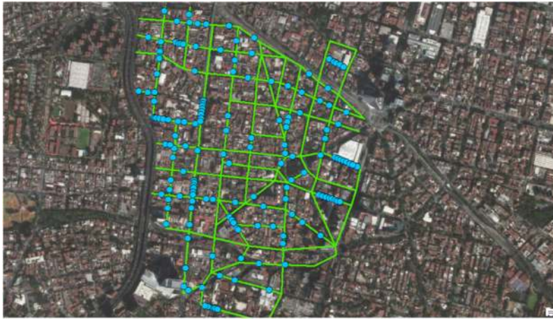
Figure 14.1 Example of a water district distribution system data. White lines represent water mains and dots reported water main failures.
