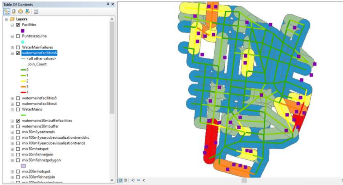
Figure 14.46 Spatial Join tool showing the number of failures per water main (refer to online version of the book to visualize colors).
