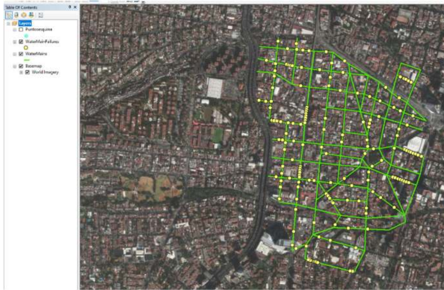
Figure 14.34 Water main grid with water main failures.
