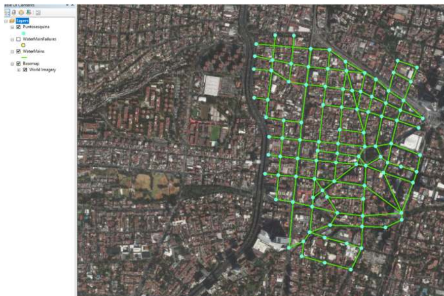
Figure 14.33 Water main grid.
