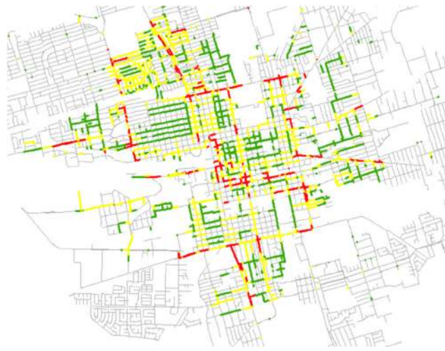
Figure 14.17 Count of critical facilities per water main. Green 0–4, Yellow 5–8 and Red 8–10 (refer to online version of the book to visualize colors).
