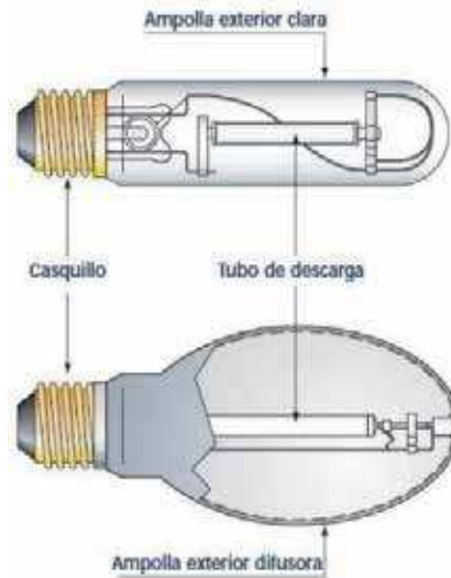
Figure 3. Parts of the high pressure sodium vapor lamp. Source: Manual INDAL lighting.
