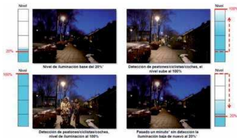
Figure 6. Dimming by motion detection.
