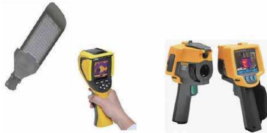
Figure 16. Experimental set-up for temperature measurement in luminaires. Source: Self made. FLUKE Ti 25 thermal camera. Source: User manual. ThermoFiguraTi25 FLUKE camera.
