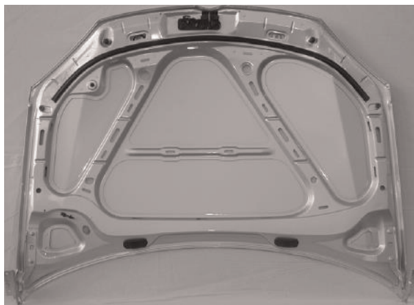
Figure 9. Hood inner panel (source of picture: Ref. [27]).
