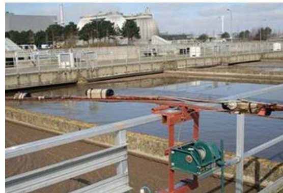
Figure 6.32: Field setup for measuring oxygen concentration profiles.
