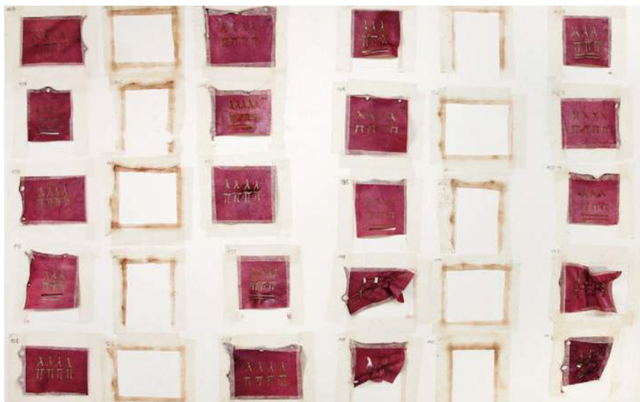
Fig. 27: The mounted samples of sub study 2 after accelerated ageing. In sub study 2 the sample set C was so deformed that the parchment pieces became detached from the mounting board.
