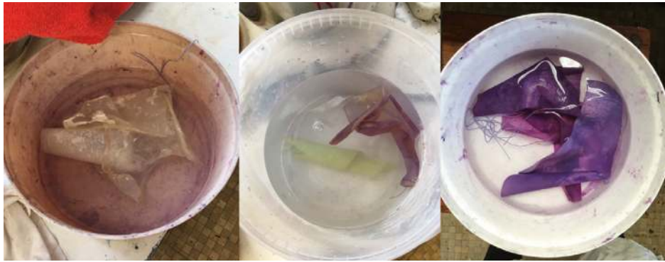
Fig. 18: a) Soaking the parchment in a mixture of vinegar and water before dyeing, b) soaking the parchment in a mixture of vinegar and water after dyeing, c) fully developed purple colour.
