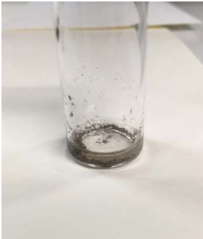
Fig. 16: Ink ST8_A in a glass. The ink could not be used for writing.
