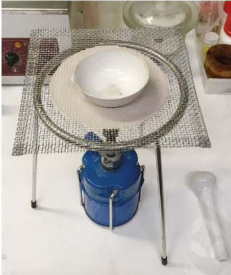
Fig. 6: Formation of an amalgam with the help of the flame of a Bunsen burner.
