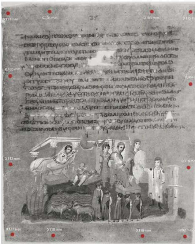
Fig. 5: Thickness measurement points, folio 18, page 35.
