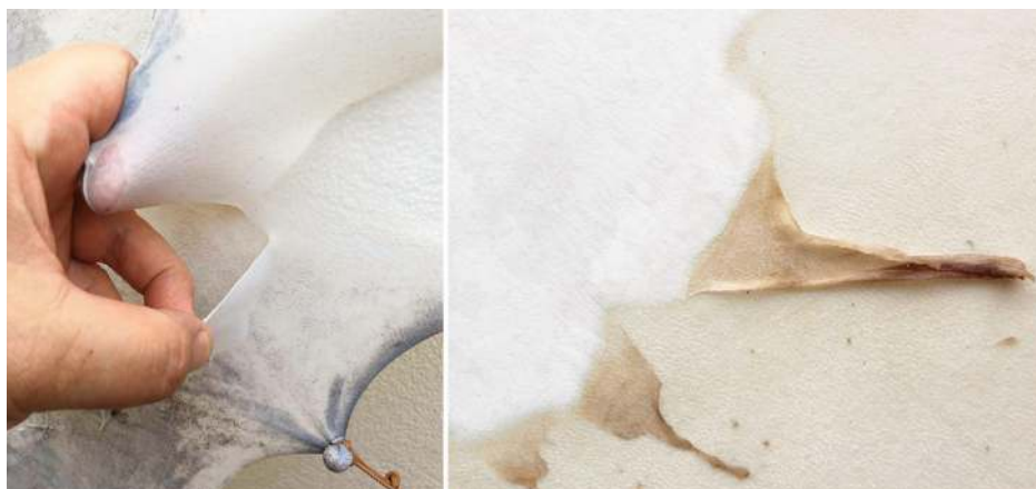
Fig. 3: On the left image, peeling off the epidermis layer on the hair side of the sheepskin; on the right image, hair side of dried sheep parchment in Late Antique style (left) and unpeeled parchment with residues of dry peeled epidermis (right).
