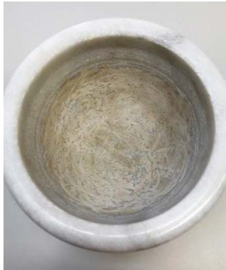
Fig. 3: Grinding silver chips together with vinegar in a mortar.
