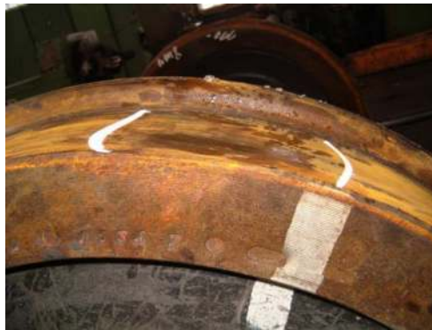
Fig. 1. Flat spot on a wheel tread 1
