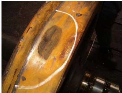
Fig. 2. Flat spot on a wheel tread 2
