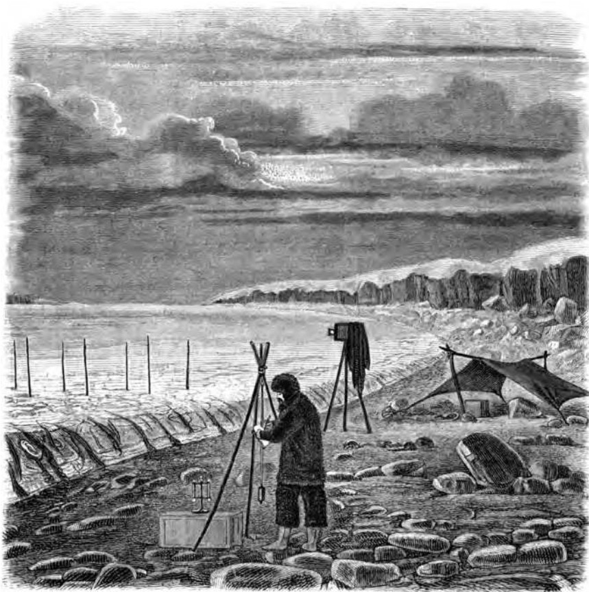
FIG. 40. Measuring glacier flow on Brother John Glacier.
