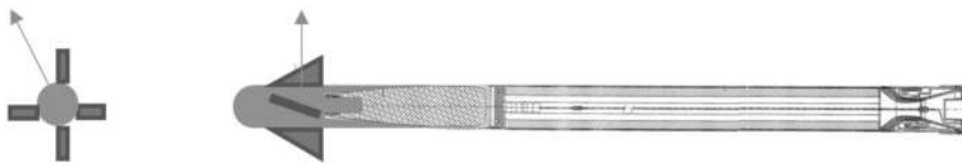
Figure 1. The 140-mm axisymmetric rocket with wrap around fins and a roll-decoupled fuse.
