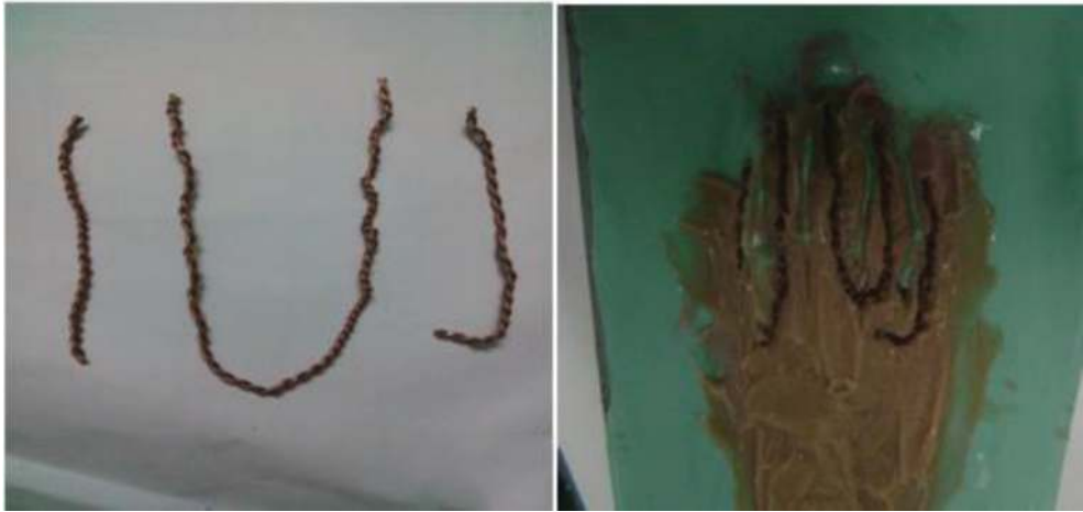
Figure 6. Copper wire and silicone die of partial hand with copper wire.
