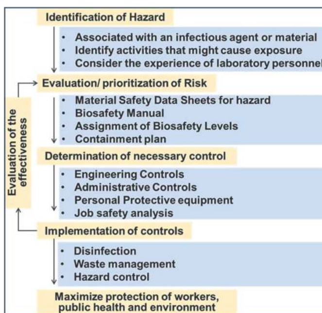
Figure 2. Flow diagram illustrating the summarizing the biosafety assessment and management process while handling cell culture-based experiments. Flow chart is inspired by reference [55].
