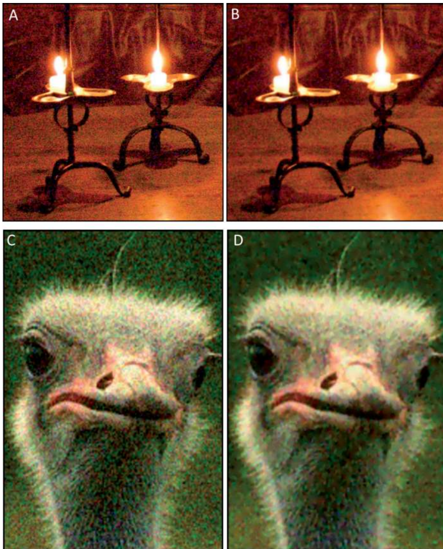
Figure 5. The NV algorithm reduced the noise level in extremely noisy color images. (A) Noisy color image of a camera taken at candle light conditions. The NV algorithm removed most noise (PSNR = 32.0 dB) (B). (C) Noisy color image of an ostrich with 10% additive Gaussian noise. (D) Noise reduced output of the NV algorithm (PSNR = 32.7 dB). Pictures printed with permission from IEEE (see Liu et al. [4]).
