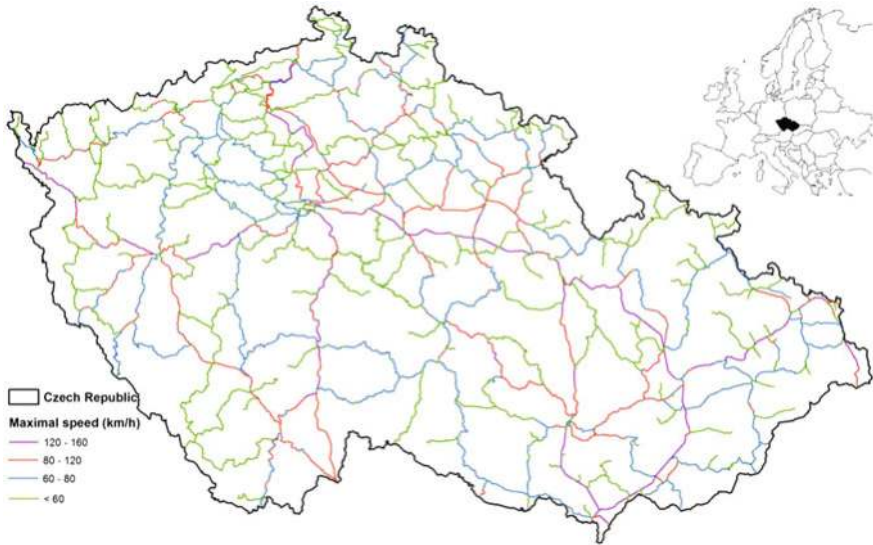
Fig. 15.2 Categorization of railways in the Czech Republic (location in Europe in inset ) by maximal speed
