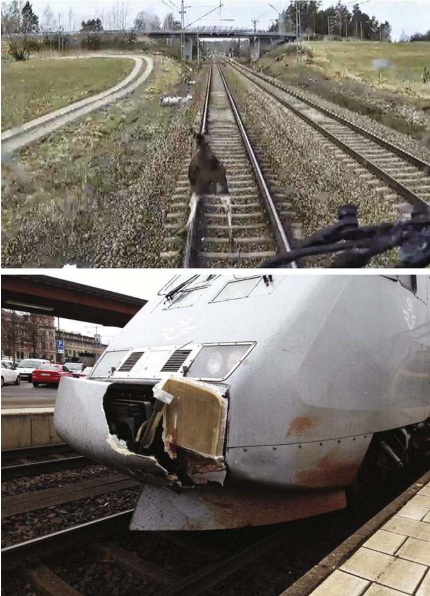
Fig. 17.4 Train driver's view of a fleeing moose shortly before collision (above). The picture was taken with a video dashcam mounted inside the driver's cabin. The damaged front of the X2000 train engine after the moose collision (below) ( photos Jimmy Nilsson, Swedish Railways )
