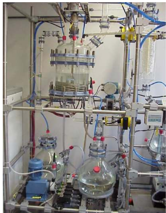
Fig. 1. The experimental pH neutralization plant.
