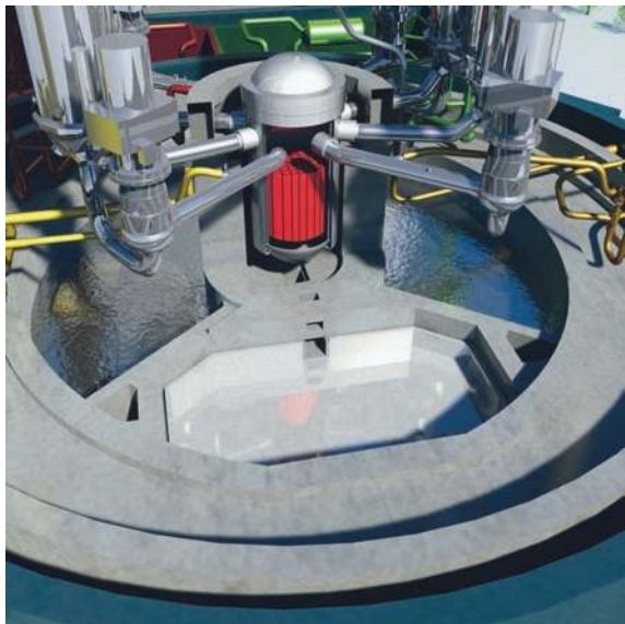
Fig. 12.18 EPR™ IRWST, spreading room and core catcher [7]
