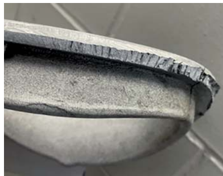
Figure 8. Fatigue crack through weld throat between reinforcement and tube.
