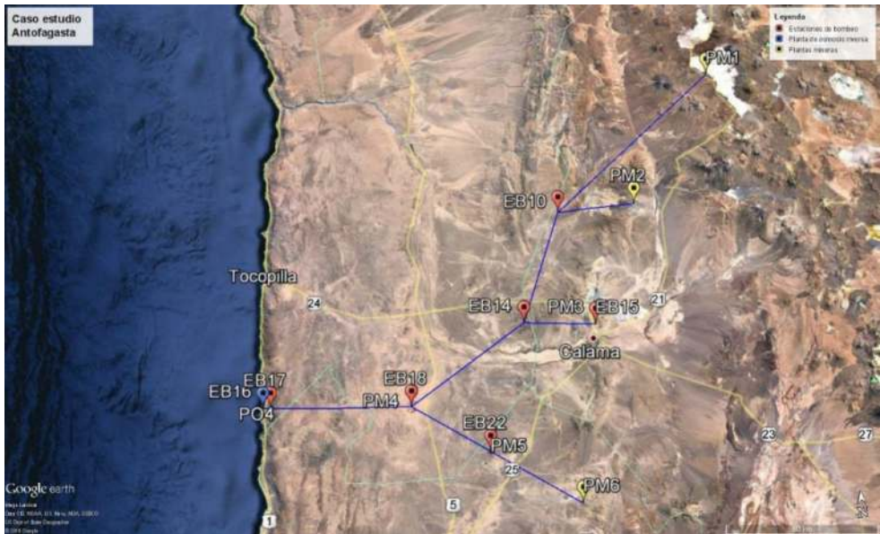
Figure 11. Optimum proposed model of an integrated desalinated water supply system for six mining plants in the Antofagasta region. PO indicator: reverse osmosis plants; EB indicator: pumping stations; and PM indicator: mining plants [14].
