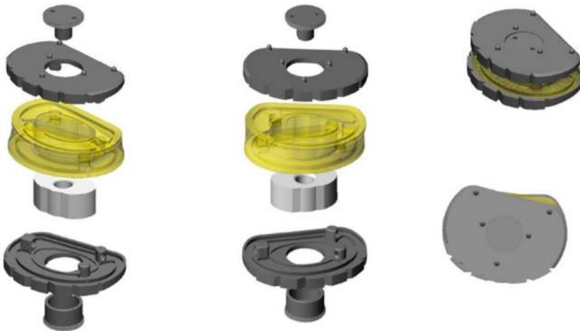
Figure 4. The geometry and position of the pegs, between the peripheral groove and the central area of the endplates, are planned to control rotational mobility
