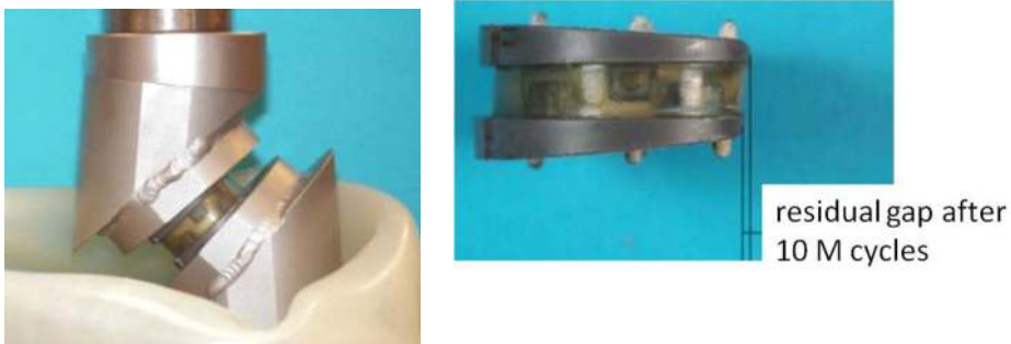
Figure 10. Wear tests were conducted in a 3-axis motion simulator (frequency = 4 Hz, loads of 135 to 1350 N), The inclination of the prosthesis was 45° to reproduce the sagittal orientation of the disk in functional situations. The gap between the metal plates was measured after each series of 10 million cycles.
