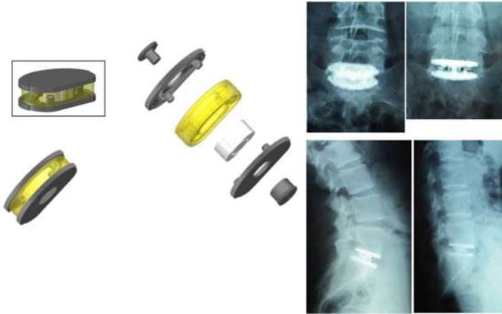
Figure 6. First generation of lumbar ESP® ( 2004 ) : endplates without lordosis
