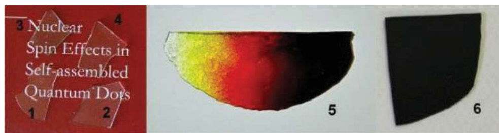
Figure 1. Photo Initial glasses doped with CdS (1), CdSe (2), PbS (3) and PbSe (4) and glasses after heat treatment doped with CdSe QDs (with different sizes) (5) and PbSe (6).
