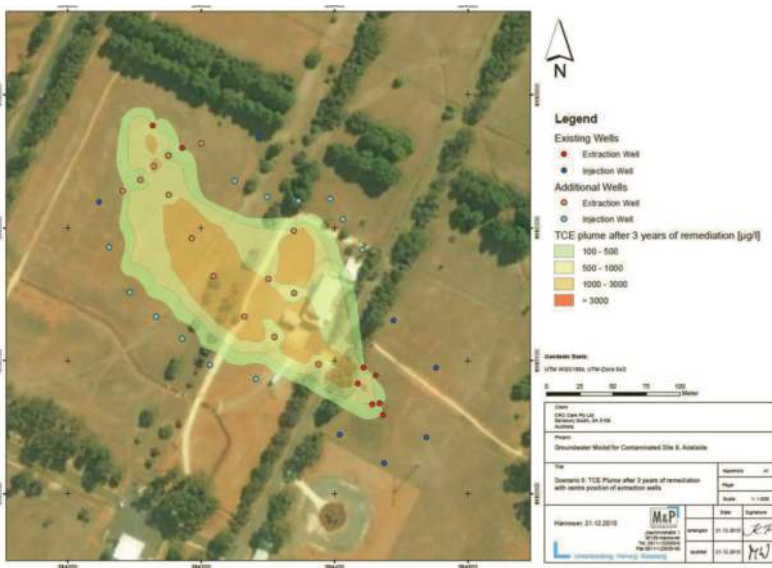
FIGURE 4.8 Simulation of TCE plume after 3 years of remediation.
