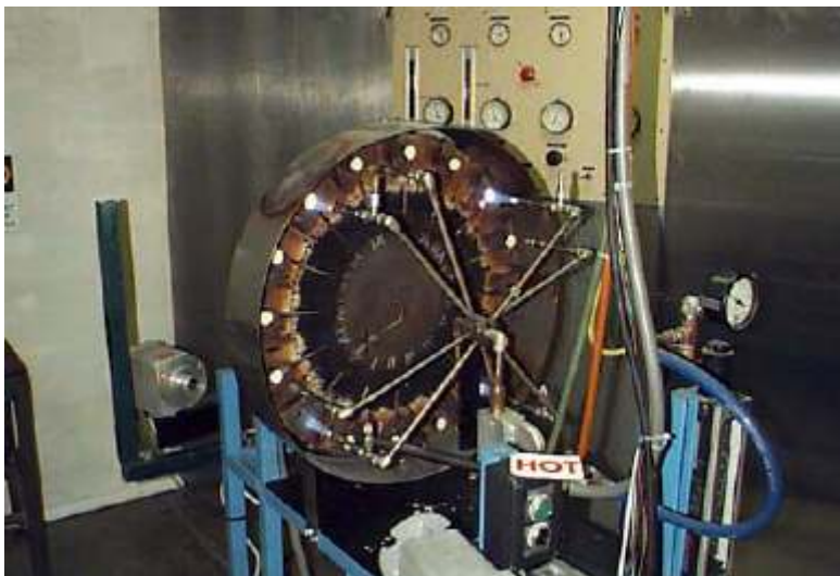
Figure 9. Wide JETS setup with four heating and cooling station [68].
