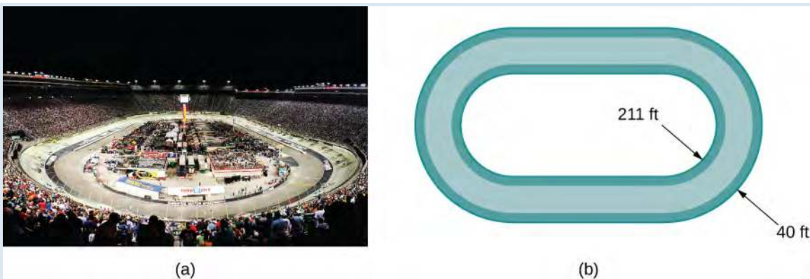
Figure 3.22 At the Bristol Motor Speedway, Bristol, Tennessee (a), the turns have an inner radius of about 211 ft and a width of 40 ft (b). (credit: part (a) photo by Raniel Diaz, Flickr)
