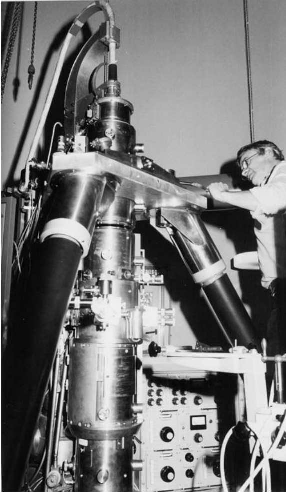
Fig. 5.7. Disassembly of the DEEKO 100 in 1996 with Klaus Weiß. One can clearly see the stabilizing tripod.
