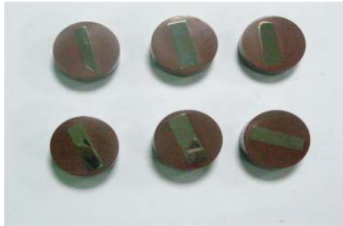
Figure 2. Digital image of the mounted samples after cutting, grinding, and polishing showing a mirror-like surface.
