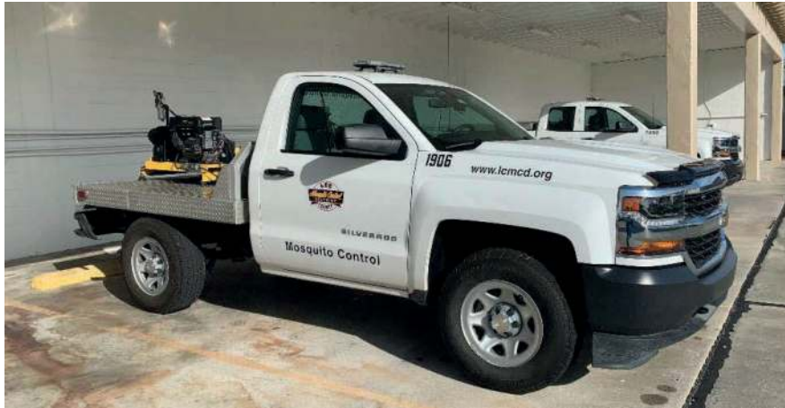
Figure 11. Ground adulticiding vehicles with rear-mounted ULV machine.
