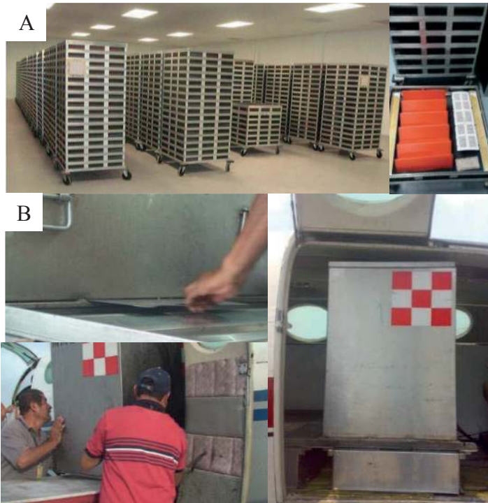
Figure 2. Towers type "México" used for the emergence of sterile adults (A) and chilled release box being loaded into the aircraft (B).
