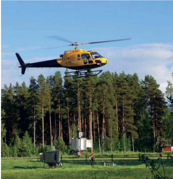
Figure 4. The use of two sling buckets, combined with change of bucket without landing the helicopter, allows for increased speed and reduced cost for aerial application of VectoBac G in the River Dalälven floodplains, central Sweden (credit J. O. Lundström).
