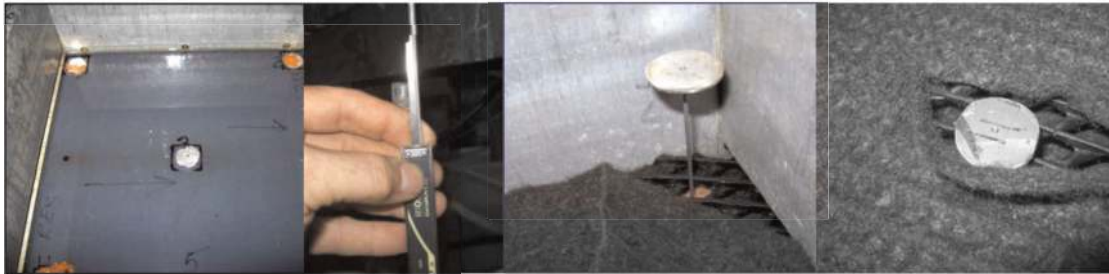
(a) Example “profiled” flow test with thickness measuring LVDT
