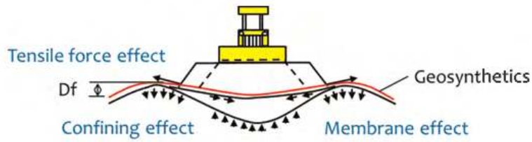
Figure 3. Geosynthetic reinforcement effects on the surface layer of a super soft soil foundation.
