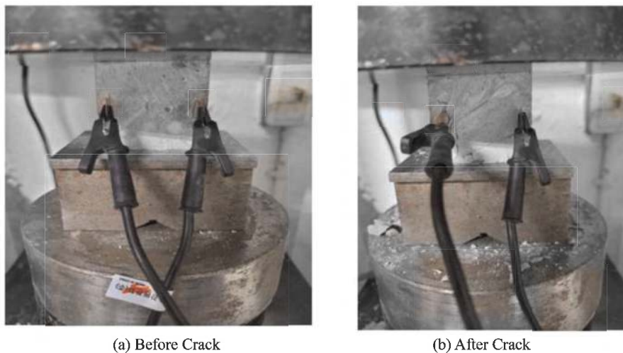
Figure 6. Method of measuring electrical resistance according to the occurrence of cracks.
