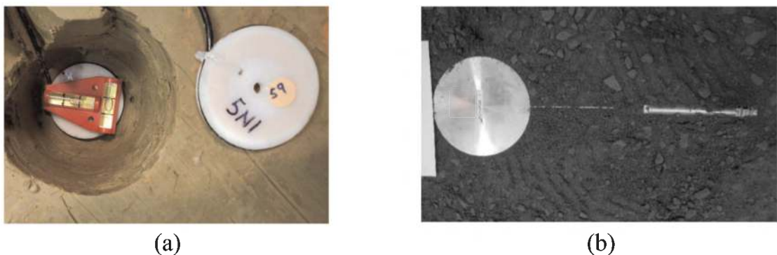
Figure 3. Embedded sensors at NAPTF CC9: (a) Inductive coil pairs, and (b) Pressure cell.
