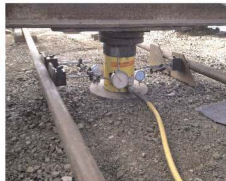
(a) Schematic cross-section of the test set-up (not to scale), “T.SPC”, “M.SPC”, and “B.SPC” indicate the location of soil pressure cells, (b) Photograph of test installation prior to loading include reaction beam, load plate, hydraulic jack and three dial gauges (Moghaddas Tafreshi et al. 2013).
