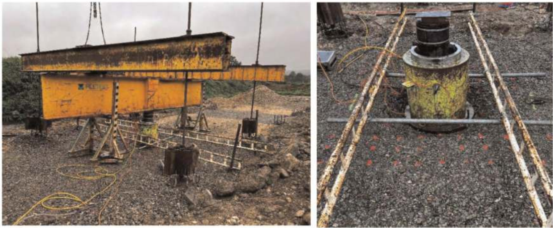
Figure 4. Left: Reaction frame; Right: Load cell.
