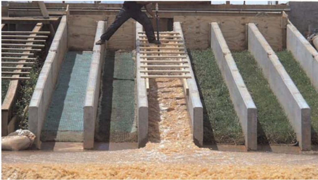
Figure 11. Large-scale channel erosion testing facility.
