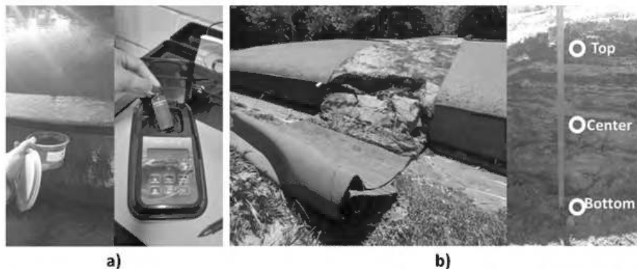
Figure 3. Sample collection. a) percolated collection, and equipment used for turbidity measurement. b) geotextile exhumation and sediment sampling.
