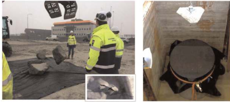
Figure 1. Examples of drop tests in the field and in a laboratory. The insert left shows an example of the damage to a geotextile. (photographs field tests courtesy of Van den Herik Contractors).
