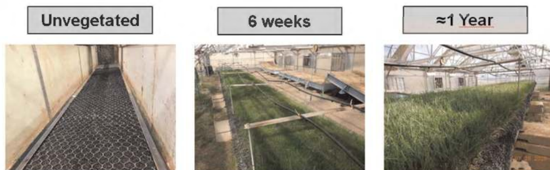
Figure 3. Pictures of Macmat 6822G0 at different vegetation growth in the CSU testing program.
