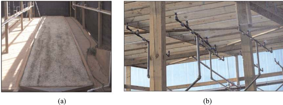
Figure 10. (a) The standard plot is a 3 to 1 slope with a down slope length of 12.2 m and a width of 2.3 m, and (b) calibrated rain delivery system.
