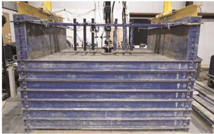
Figure 5. Cyclic plate load test apparatus (courtesy of TRI Environmental, Inc.).
