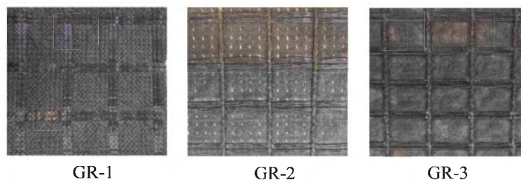
Figure 2. Polymeric Geosynthetic Reinforcements evaluated in the study: a) GR-1; b) GR-2; and (c) GR-3.
