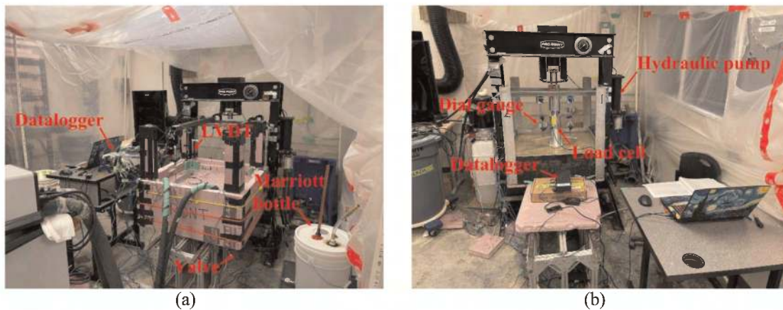
Figure 2. Photographs: (a) freeze-thaw tests and (b) plate loading tests.
