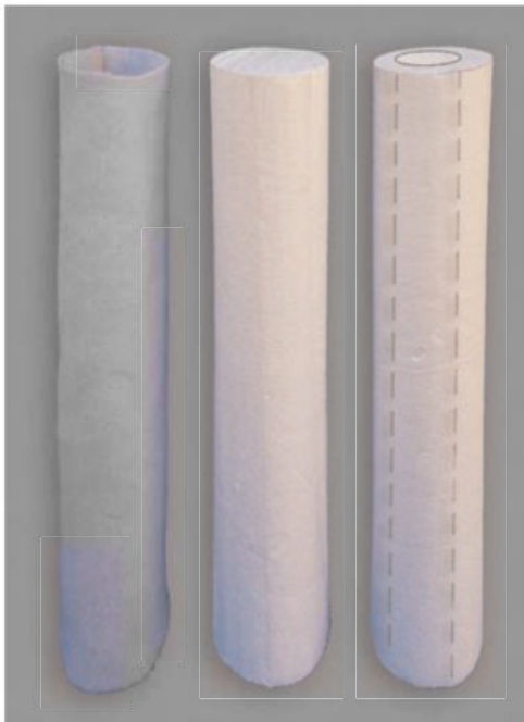
Figure 1. Reinforcement materials: (a) Hollow Geofom, (b) Normal Geofom, (c) Geotextile.
