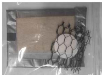
Figure 1. Filter paper setup for measuring total suction.
