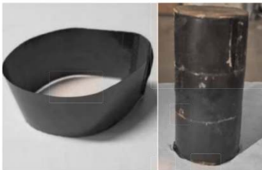
Figure 1. Geocell and the reinforced silty clay specimen.
