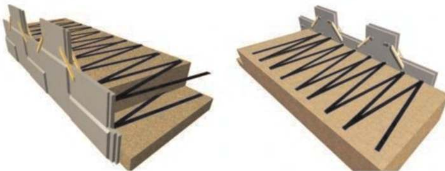
Figure 2. Typical of geoforce segmental retaining wall system.
