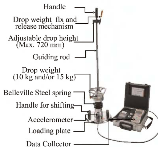
Figure 2. Schematic view of Light Weight Deflectometer (LWD) NDT Device and its components.
