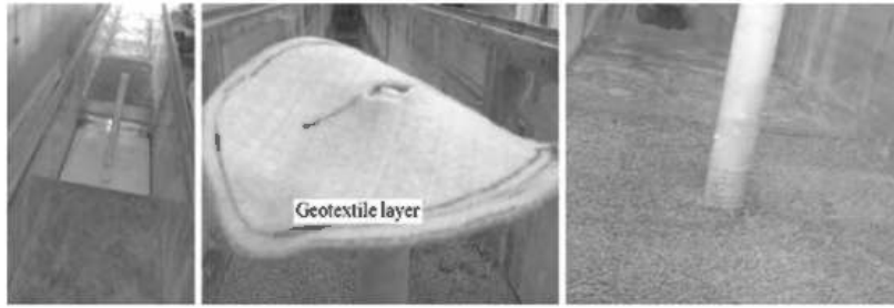
Figure 3. Photographs of experiments using a geotextile collar as a pier scour countermeasure (Nouri Imamzadehei et al. 2016).
