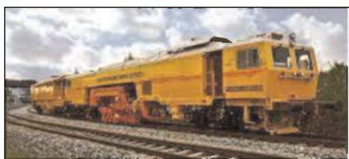
Figure 18(a). Dynamic tamping express machine.
