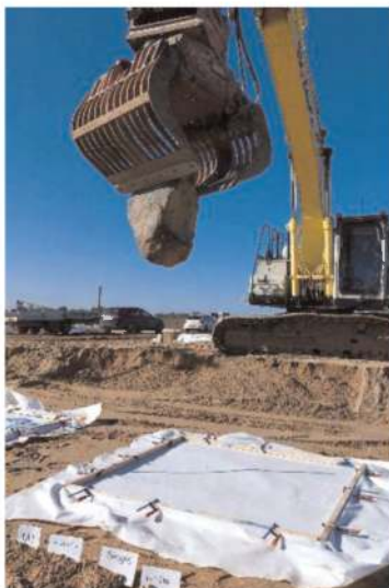
Figure 8. Fieldtrial drop tests with selected stone classes on nonwoven geotextile and analysis of failure mechanism and test conditions subsoil.
