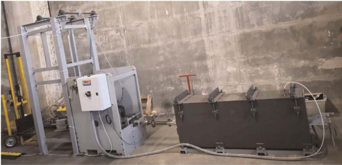
Figure 11. Large-scale prototype apparatus for long-term pullout tests.
