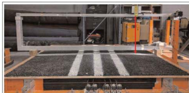
Figure 4. Profilometer mounted on the section (Highlighted in green is the laser distance meter).
