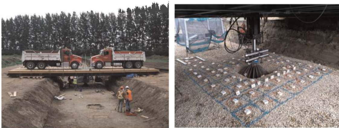
Figure 1. Saskatchewan University full scale temporary working platforms testing (Left: general set up, right: platform after the test).
