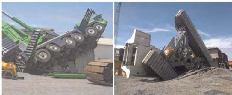
Figure 1. Examples of construction machinery overturning.
