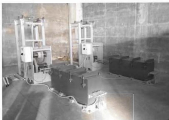
Figure 1. Large-scale prototype apparatus for long-term pullout tests.
