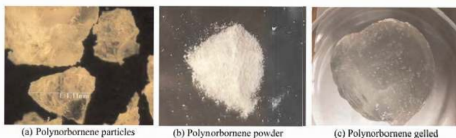
Figure 2. The organic pollutants absorption and gelation behavior of polynorbornene resin.
