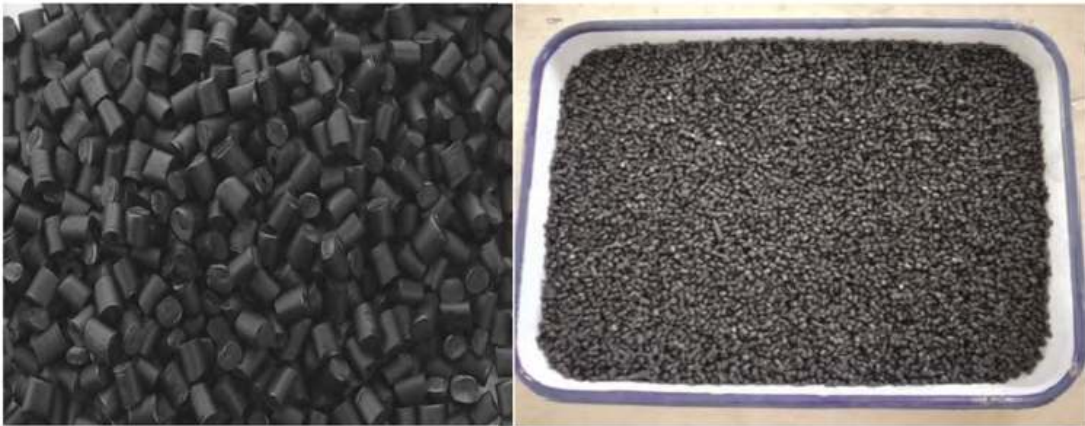
Figure 1. Raw material of electrically conductive polymer with resistivity of 10^{-3}\Omega\cdot\text{m} .
