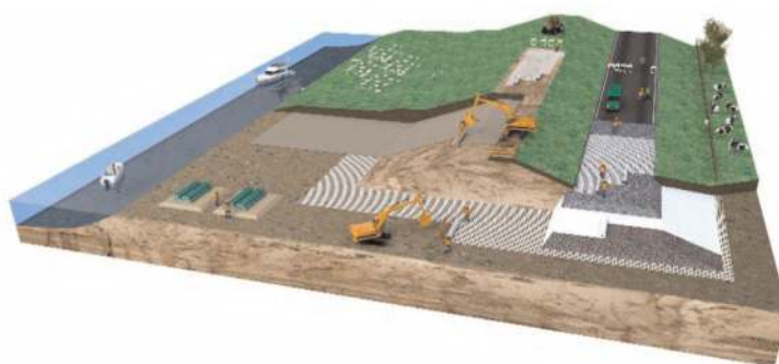
Figure 4. Systematic section of a high-performance flood defence construction with soil reinforcement, geosynthetic clay liner as a barrier, nonwoven geotextile for filtration and separation and erosion control products on the embankments.
