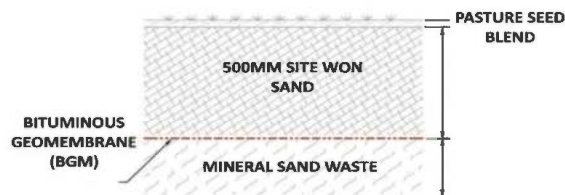
Figure 2. Schematic of mineral sand waste capping solution.
