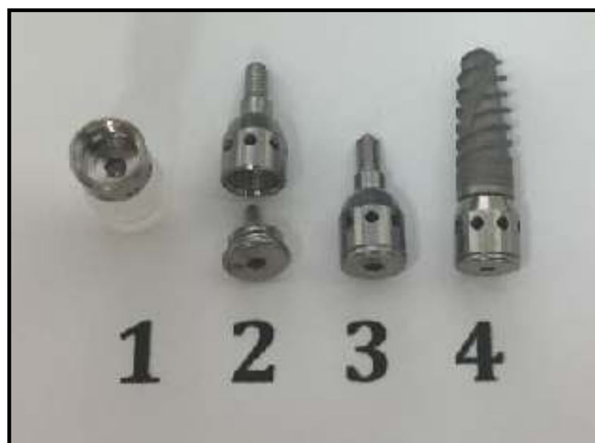
Fig. 3. Bioactive healing abutment structure and dental implant fixation
