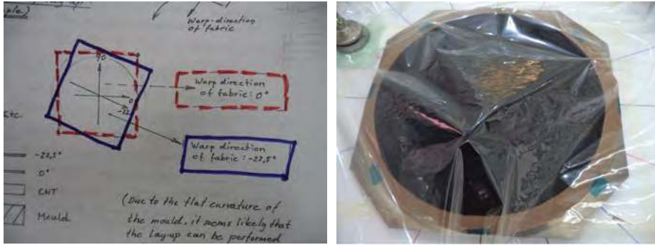
Figure 4.14: CNT-BP facing the mold.
