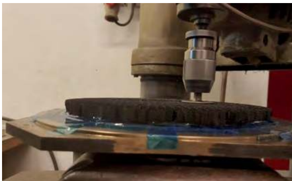
Figure 4.24: Honeycomb machining to obtain a flat surface.
