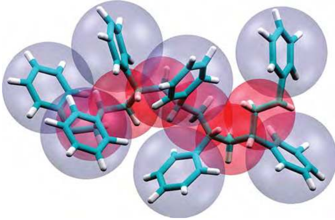
Figure 3.18: Coarse-grained model of polystyrene (red and gray beads) from atomistic details (white and cyan sticks). Reprinted from Ref. [139] with permission of American Chemical Society.
