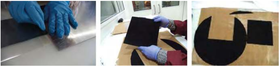
Figure 4.12: Cutting the CNT-BP with the proper size.
