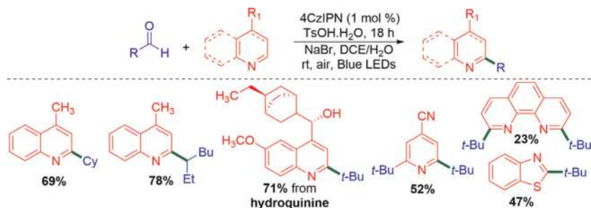
Figure 21. 4CzIPN-photocatalyzed decarbonylative Minisci reaction.
