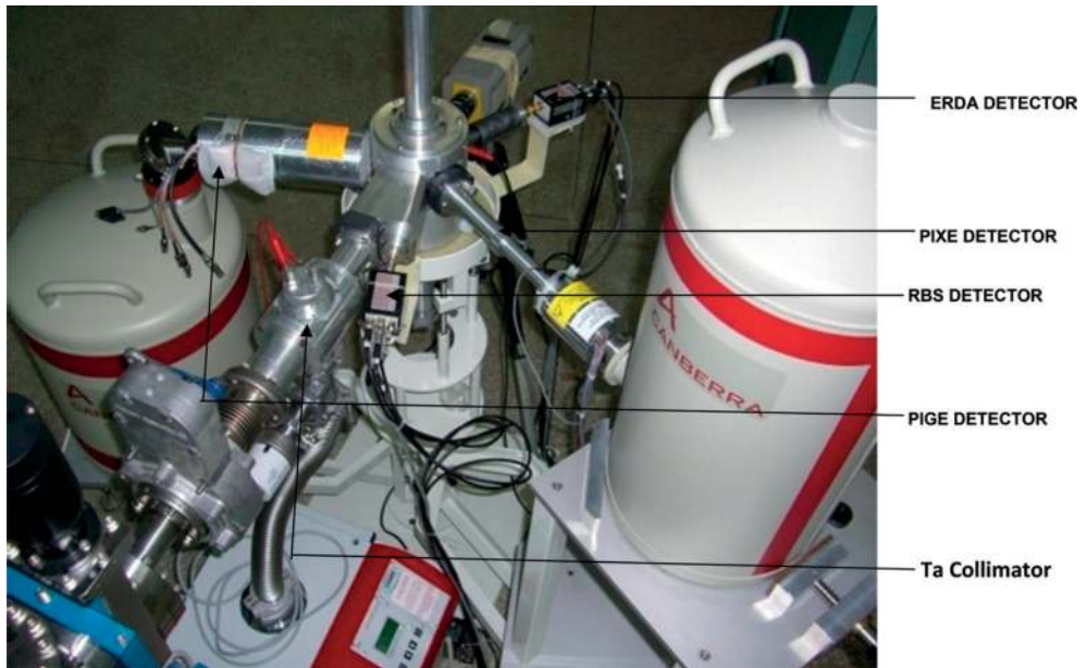
Figure 3. General view of the IBA End Station at CERD, OAU, Ife, Nigeria showing four ports and a window for RBS, PIXE, ERDA, and PIGE detectors (Source: [13]).
