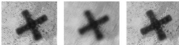
Figure 4. Cross-target images: original image without aberration applied (left), with aberration applied and AO off (center), with aberration applied and AO on (right). 9x9 lenslets (without those on the four corners) are used for wave-front sensing, and 25 Zernike modes are corrected.
