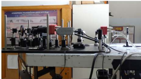
Figure 5. PSAO setup (the black breadboard) on the McMP rotation station. The two red cameras are used for WFS and TTS, while the grey one is the science camera.
