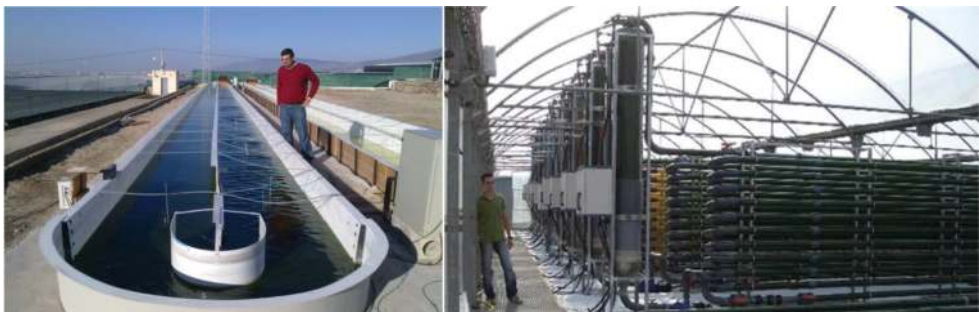
Figure 4. Image of some photobioreactors used for outdoor production of microalgae at a large scale. A raceway reactor of 20 m 3 as an example of open reactor (left side) and ten tubular reactors of 30 m 3 as an example of tubular reactors (right side). All of them installed and operated at Estación Experimental Las Palmerillas (Fundación Cajamar), Almería, Spain.
