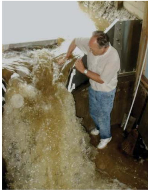
Figure 5. Turbulent flow in a NAEW drop-box weir for flow measurement in sediment-laden runoff.
