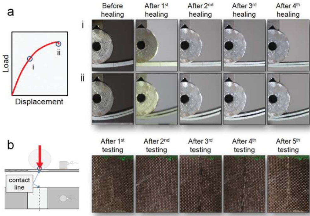
Figure 19. (a) Snapshot during the mode II interlaminar fracture toughness testing of the modified CFRP (i) just after crack propagation onset and (ii) just before failure (i.e. P \sim P_{\max} ), before and after healing. (b) Photographs showing the progressive damage accumulation on the upper layers of the modified CFRP during the mode II testing, with increasing the number of testing cycles. The damaged line is the contact line between the specimen and the loading cylinder.
