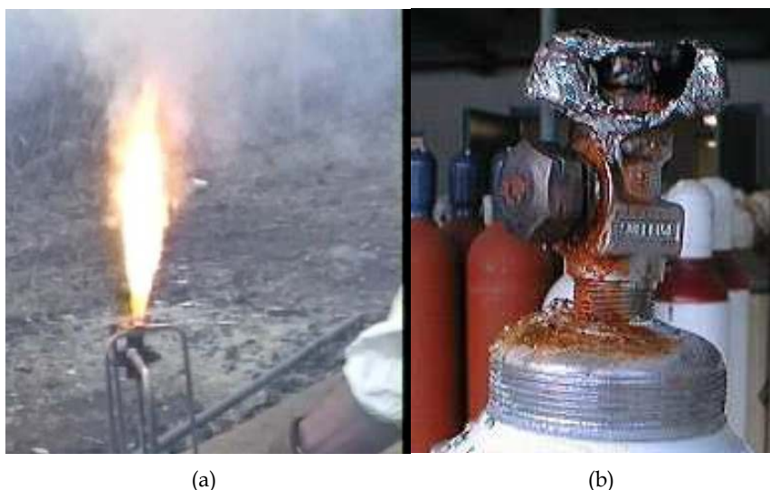
Fig. 3. Typical phosphine combustion flame and powder. (a) Orange flame and white phosphorous pentoxide powder (b) Red phosphorus powder.
