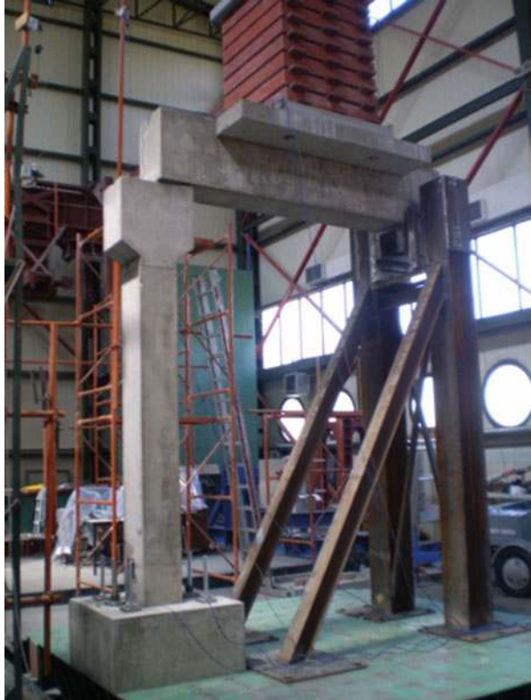
Fig. 4.30 Shake table test of the beam-to-column dowel connection at NTUA
