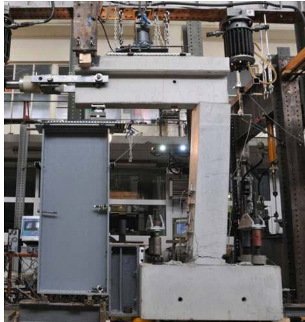
Fig. 4.29 Test of the dowel connection at large relative rotation between the beam and column
