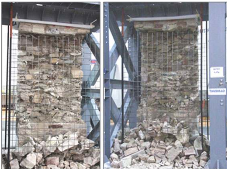
Fig. 8.19 Failure of walls 1 and 2 (Valluzzi et al. 2013)
