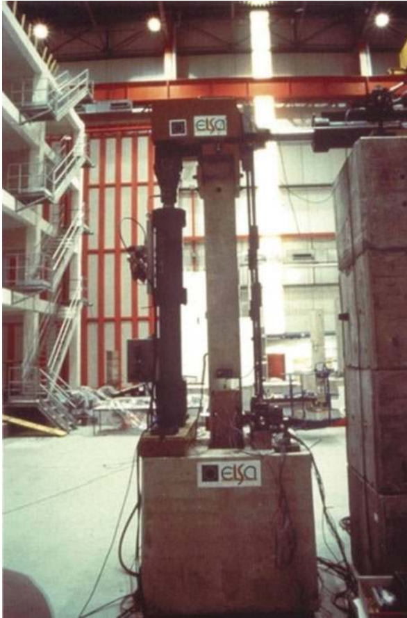
Fig. 4.16 ASSOBTETON tests on precast columns with pocket foundation performed at ELSA
