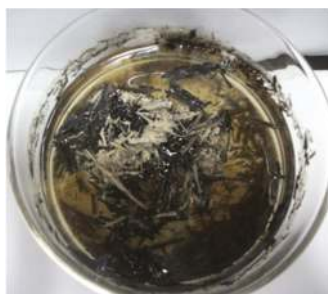
Figure 9. A bitumen sample in Instant ocean treated with CaO-coated charred hay sample at room temperature (23 °C) and time = 336 h.
