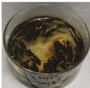
Figure 8. A bitumen sample in Instant Ocean treated with charred hay at room temperature (23 °C) and time = 288 h.
