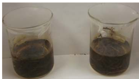
Figure 7. Bitumen samples with charred hay (60 min) added in deionized water (right) and Instant Ocean solution (left) at room temperature (23 °C) and time = 186 h.
