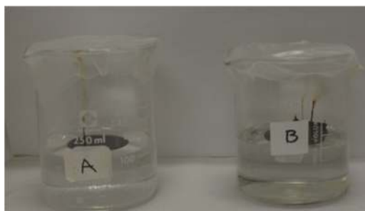
Figure 4. Bitumen samples in deionized water (A) and Instant Ocean solution (B) at room temperature (23 °C) and time = 0 h.
