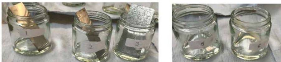
Figure 3. Sample of qualitative soaking test carried out to identify potential material incompatibilities with neat octanol. Sample 1, stainless steel; Sample 2, steel; Sample 3, galvanised steel; Sample 5, PVC hose; Sample 6, PTFE hose. Besides a slight swell of the PVC pipe, no material alterations were observed.
