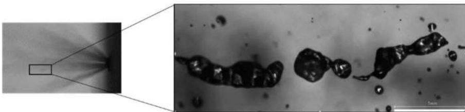
Figure 4. LN 2 spray into ambient air. The left image shows the spray in whole. The right image is the magnified image of the location marked by black rectangle in the whole spray.
