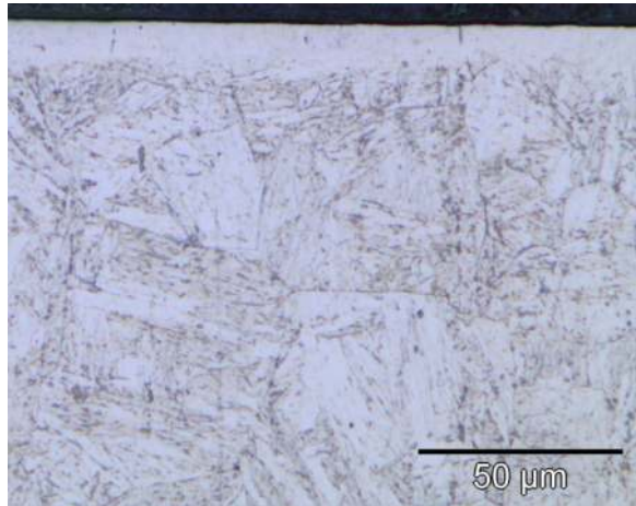
Figure 5. Cross-sectional micrograph of a low-temperature nitrated AISI 420, treated at 350°C for 4 h.
