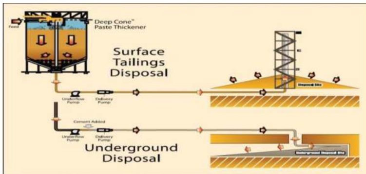
Figure 14. Paste thickening of treated neutralized effluent in the Coal mining AMD.
