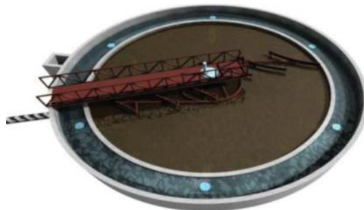
Figure 5. The thickener clarification of AMD water in the Simak Coal Mine Site for fishery pool remediation e - .
