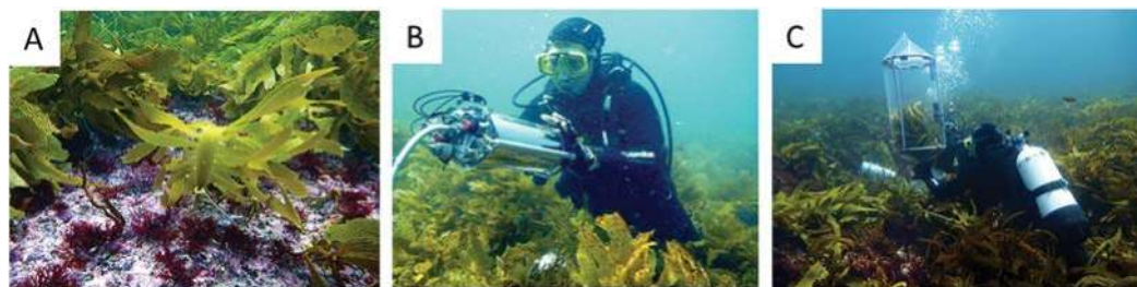
Figure 4 Measurements of Ecklonia radiata growth and productivity can be taken using methods including (A) tagging plants and ‘hole-punching’ to measure growth of the primary blade, which can be converted to biomass accumulation, (B) Pulse amplitude modulated (PAM) chlorophyll fluorescence to measure the rate of transport of electrons through photosystem II, which is increasingly used as a proxy for gross photosynthesis and (C) photorespirometry chambers to measure oxygen metabolism. (All photographs by the authors.)
