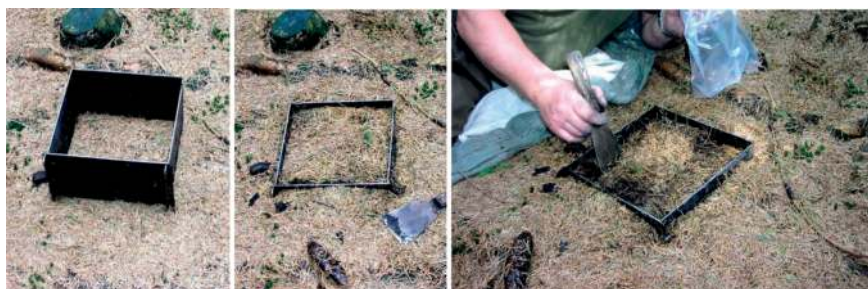
Figure 1. Sampling of forest floor L layer using steel frames (25 × 25 cm) in Norway spruce stands.
