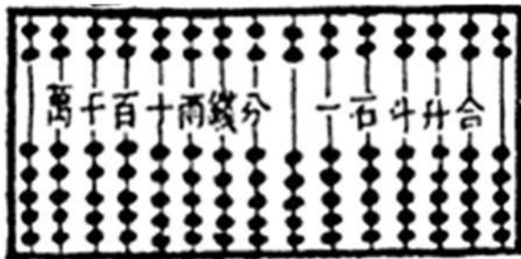
Fig. 3.3 An ancient drawing of a suàn pán (算盘) with measurement units ( https://commons.wikimedia.org/wiki/File:Ming_suanpan.JPG )
