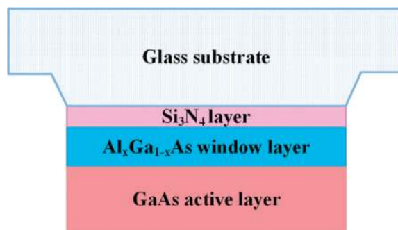
Figure 3. Structural schematic of multilayered t-mode GaAs cathode module, including the glass substrate, the \text{Si}_3\text{N}_4 antireflection layer, the \text{Al}_x\text{Ga}_{1-x}\text{As} window layer, and the GaAs active layer.
